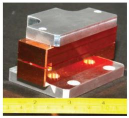
Figure 3: SLAC open mm-wave travelling wave accelerating
