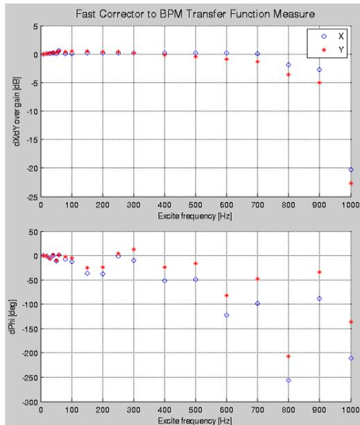
Figure 5: Amplitude and phase response for C01 fast corrector #1. Amplitude response was calculated from PSD spectrum and phase response from I-Q detection method.
