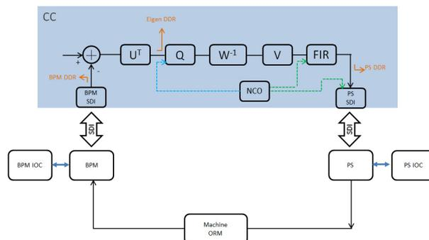
Figure 1: Schematic of NSLS-II BPM, CC and PS. FOFB signal processing is implemented in the CC where a NCO is available to drive the fast corrector. Similar NCO function can also be generated inside the BPM electronics.
