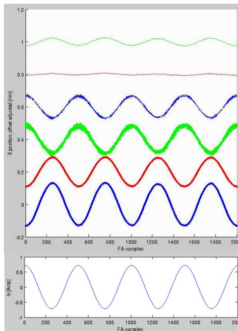
Figure 3: Time domain beam orbit response when one corrector was exciting the beam at 20Hz. C30 six BPMs X position FA data is plotted together with the fast corrector current waveform in the bottom.
