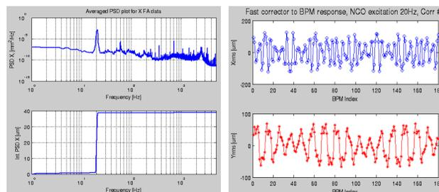
Figure 4: (Left) PSD spectrum while beam was excited by one fast corrector with driving frequency of 20Hz. (Right) RMS motion around the excitation frequency was calculated from the PSD spectrum at BPMs around the ring.
