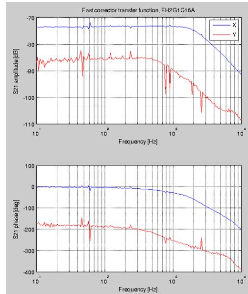
Figure 6: Amplitude and phase transfer function measured with tune system network analyzer.
