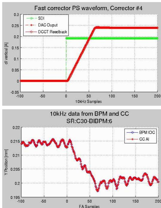
Figure 2: Fast corrector to BPM setup response. (Upper) green - Fast corrector setting value from CC NCO; red – power supply received data and readback current. (Lower) BPM 10kHz data from IOC and CC.
