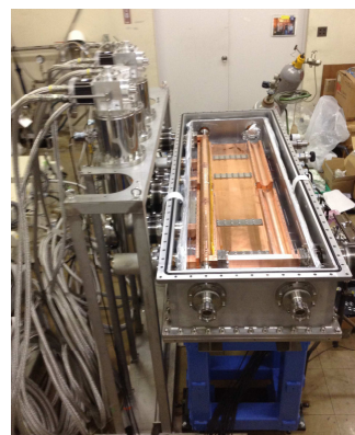
Figure 9: The cryostat for cooling the accelerating structure.
