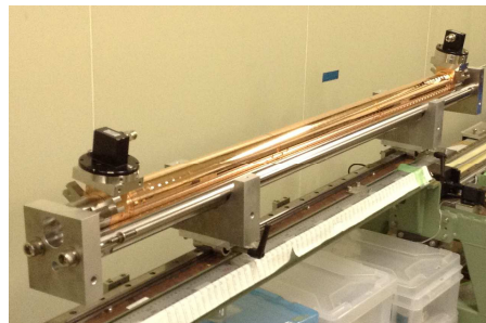
Figure 8: The accelerating structure during low-power test at room temperature.
