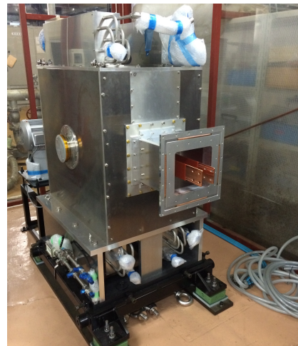
Figure 4: An air-cooled cavity for the second harmonic RF. The air flows from the inside of cores to the outside. The warm air will be cooled by heat exchanger located to the upper and lower of the cavity. The air will circulate between the blower and cavity.
