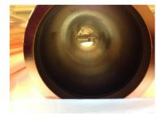
Figure 3: TiN coating of the inner suface of coax waveguide.
