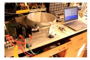
Figure 10: Actuator lifetime test.
