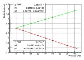
Figure 9: Actuator functional test: Deflection vs Applied pressure.
