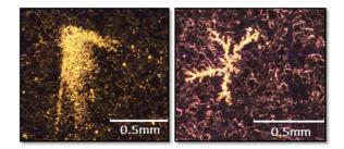
Figure 4: Typical cavity damage observed after high-power B=0T run.
