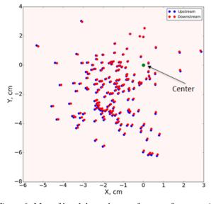
Figure 6: Map of breakdown damage from a reference point of downstream endplate, upstream coordinate are flipped in X. Red and blue dots correspond to pits on the opposing flat walls.
