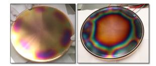
Figure 3: Interior surface of endplates. The variation in coloring is due to difference in TiN coating thickness.
