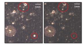
Figure 7: Copper "splashes" observed after B=3 T run (left) and the same region (right) after the subsequent B=0 T conditioning run. Disappearance of spots is highlighted.
