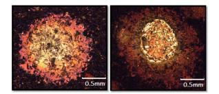
Figure 5: Microscopic images of typical breakdown "pits" with and without melted core present.
