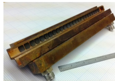
Figure 2: Vacuum dry load with AlN ceramic wedges.
