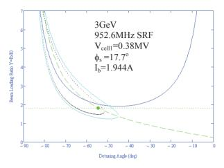
Figure 7: Robinson diagram showing working point with A=1,  $\tau_d=0.4\mu$ s, and contours for  $P_{for}=260$ kW (black dotline) and  $P_{for}=280$ kW (cyan solid-line).
