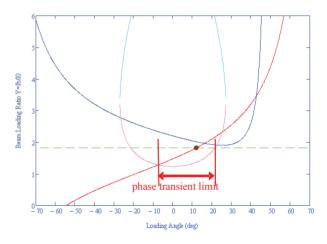
Figure 8: Pedersen diagram showing the estimated beam synchronous phase transient limit. Klystron power contour line (magenta) is for 280kW. Other parameters are same as in Figure 7.
