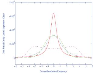
Figure 6: Real part of cavity impedance: red solid, A=0; blue dot-line, A=1,  $\tau_d=0.4\mu$ s; green dash-line, A=1,  $\tau_d=0.8\mu$ s; magenta dot-dash-line, A=4,  $\tau_d=0.4\mu$ s. All input parameters are same as in Figure 5.
