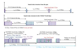
Figure 2: Time structure of electron bunch trains from injector gun to CEBAF and then to Figure-8 electron ring.
