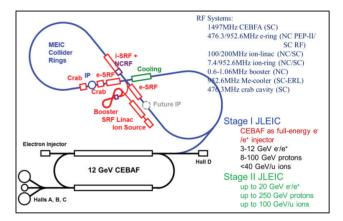
Figure 1: Layout of conceptual design of staged JLEIC with NC and SC RF systems.
