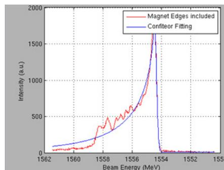
Figure 2: Maximum LINAC operating energy.
