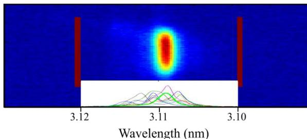
Figure 5: Single shot spectrum at harmonic  $17 \times 5 = 85$ .
