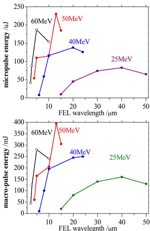
Figure 2: The MIR-FEL performance from simulation. **Top:** micro-pulse energy; **Bottom:** macro-pulse energy with the micro-bunch repetition rate of 238 MHz.
