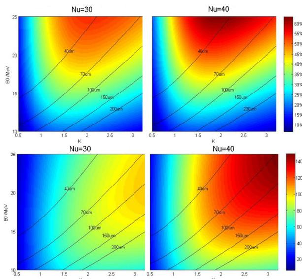
Figure 3: The small signal gain for the FIR-FEL with different undulator lengths. **Top:** with no waveguide; **Bottom:** with planar waveguide ( $b=10$  mm).
