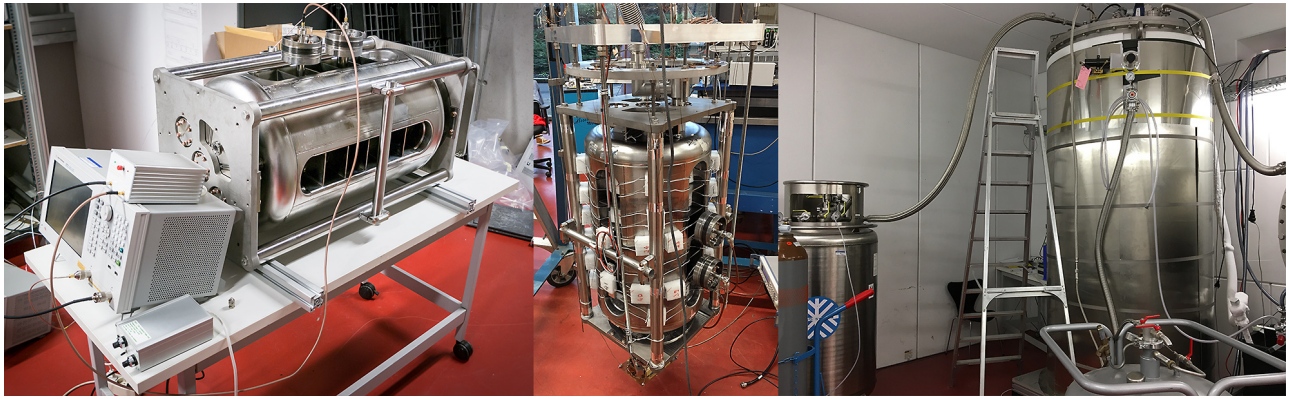
Figure 5: Frequency measurement on the 15-gap CH cavity ( left ). Thermoluminescent dosimeters (TLDs) were mounted around the cavity for field emission measurements ( center ). Conditioning and power tests were performed at IAP with a vertical cryostat ( right ).
