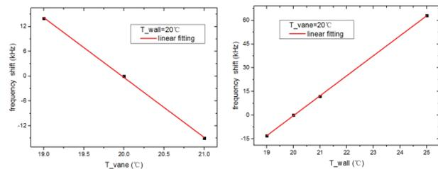
Figure 9: Temperature frequency sensitivities for vane (left-9(a)) and for wall (right-9(b)).
