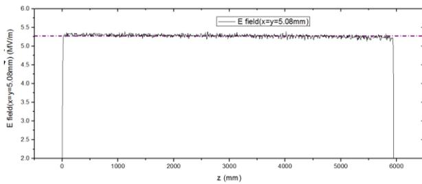
Figure 6: Electric field amplitude distribution along line in the gap between vane tips.
