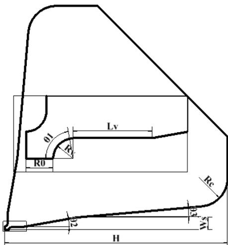
Figure 2: Cross-section geometry of LEAF-RFQ.
