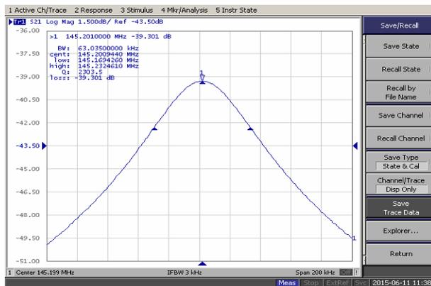
Figure 3: The operating frequency of 145.2 MHz is tuned.
