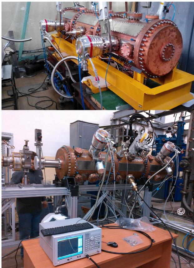
Figure 6: RFQ linac with RF and vacuum components installed on resonator in tuning area at ITEP (top) and linac with laser ion source in Nuclotron injector's hall at JINR.
