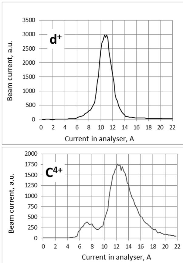
Figure 8: Measured spectrums for accelerated deuterium (top) and carbon  $C^{4+}$  beams.
