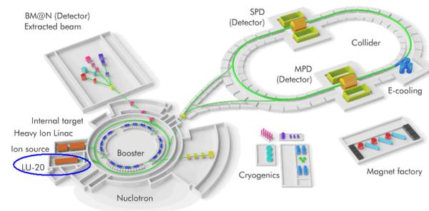
Figure 1: NICA complex. Proton, light and polarized ion linac LU-20 with new RFQ injector is marked.
