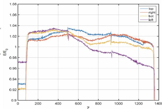
Figure 4: RF field amplitude deviation (< 2%) in four quarters of RFQ resonator.
