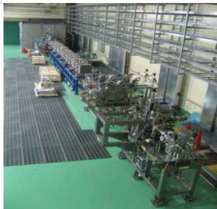
Figure 2: View of LIPAc in Rokkasho with its D-plate, MEBT, the 9.7 m long RFQ and Ion source + LEPT.
