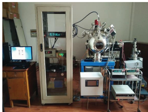
Figure 2. SEY test device.
