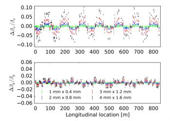
Figure 1: Simulated  $\beta$ -beating of single particles tracked through the nominal lattice with the nominal model used for reconstruction by N-BPM method, with transverse displacement at  $\beta_x = 36$  m and  $\beta_y = 6$  m as shown in the legend (notation: horizontal x vertical).
