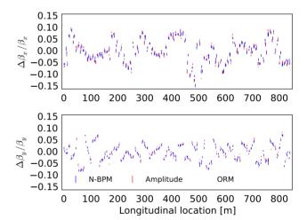
Figure 2: Measured  $\beta$ -beating with respect to the nominal model obtained by three different methods: N-BPM, Amplitude and ORM.
