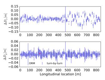
Figure 4: Dispersion deviation from the nominal model obtained from ORM and turn-by-turn data.
