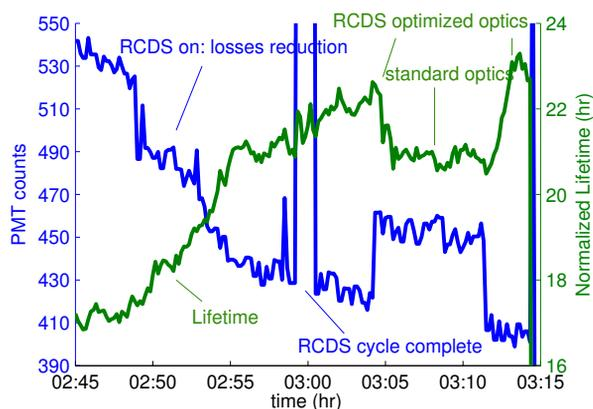
Figure 3: Change in normalised lifetime and loss-rate as a function of RCDS iteration number. The effect of switching between initial and optimised sextupoles is highlighted.
