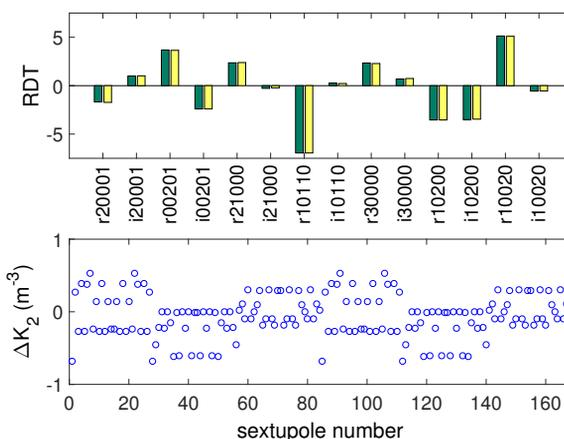
Figure 4: Top: RDTs before (green) and after (yellow) optimisation. Bottom: Associated change in sextupole strength.
