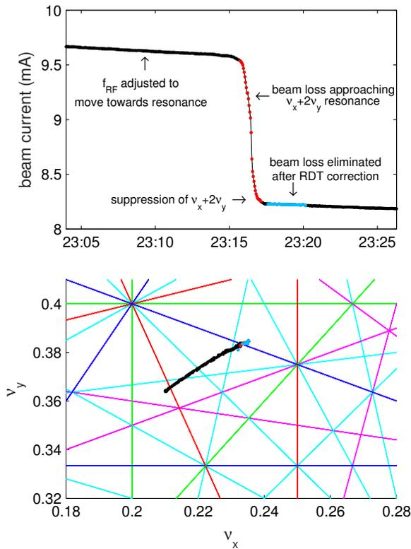
Figure 1: Suppression of the  $\nu_x + 2\nu_y = 54$  RDT (see text for further explanation). Top: beam current as a function of time. Bottom: measured tune during the optimisation.
