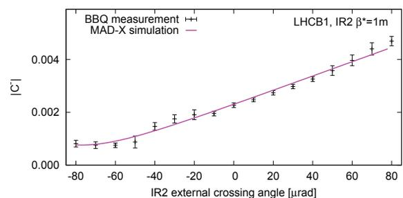
Figure 2: Modelled and measured change of  $|C^-|$  with vertical crossing angle in the ALICE IR ( $\beta^* = 1$  m).
