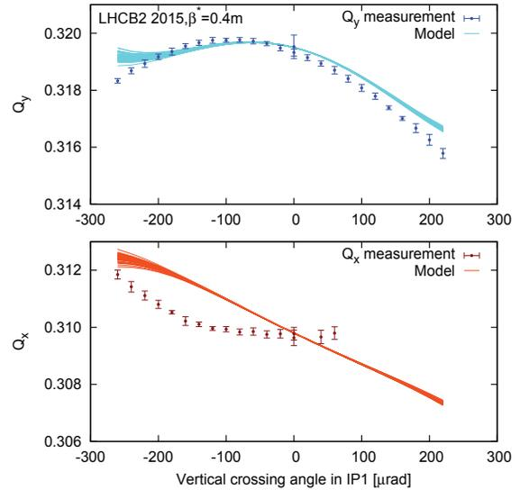
Figure 4: Modelled and measured change of  $Q_{x,y}$  with vertical crossing angle in the ATLAS IR ( $\beta^* = 0.4$  m).
