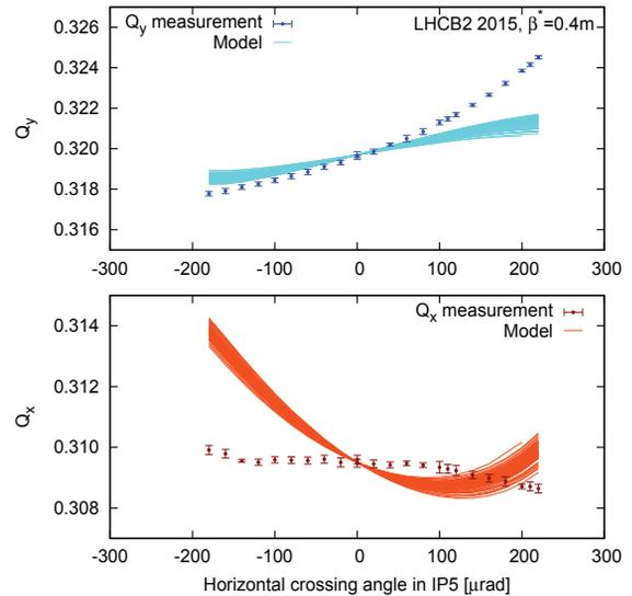
Figure 5: Modelled and measured change of  $Q_{x,y}$  with horizontal crossing angle in the CMS IR ( $\beta^* = 0.4$  m).
