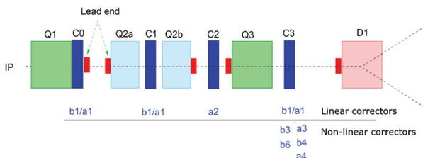
Figure 1: Corrector layout in LHC experimental IRs [2].
