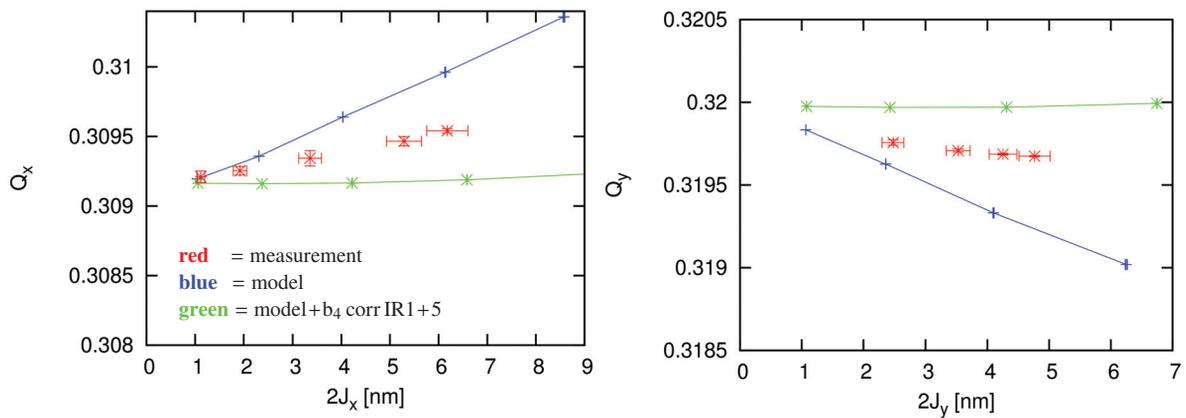
Figure 6: Modelled and measured amplitude detuning ( $\beta_{IP1,5}^* = 0.4$  m).
