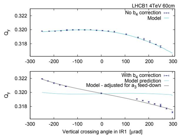
Figure 7: Effect of  $b_4$  correction at  $\beta^* = 0.6$  m on  $Q_y$  of LHC Beam 1.
