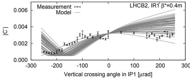
Figure 3: Modelled and measured change of  $|C^-|$  with vertical crossing angle in the ATLAS IR ( $\beta^* = 0.4$  m).
