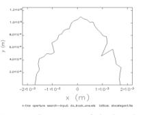
Figure 2: Dynamic aperture of the bare lattice of the JLEIC ion collider ring at IP.
