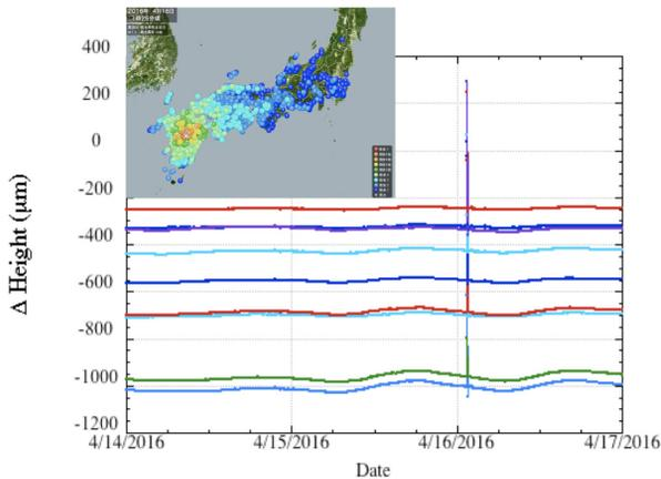
Figure 8: Floor level jump caused by the earthquake.
