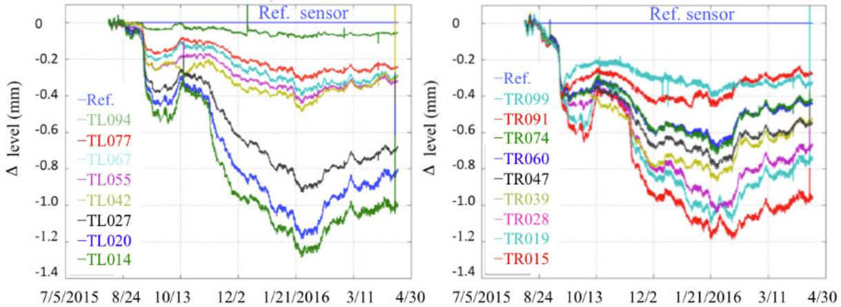
Figure 2: Floor level change at the left side of the IP (left) and the right side of the IP (right) are shown. Floor level with respect to the reference HLS unit has been plotted, beginning from August 2015.
