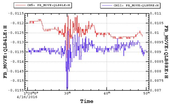
Figure 10: The variation seen in the displacements between two adjacent magnets.
