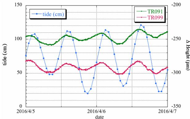
Figure 5: Tidal data compared with the tunnel motion.
