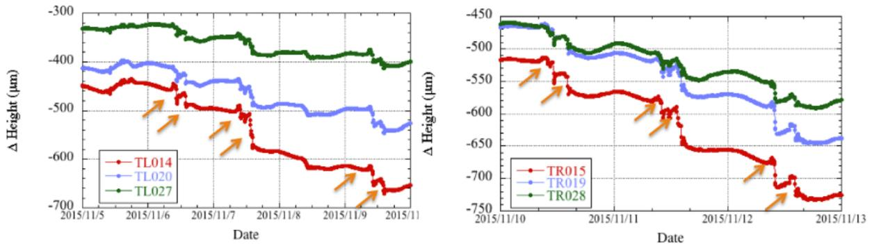
Figure 7: Level change due to the radiation shield installation.
