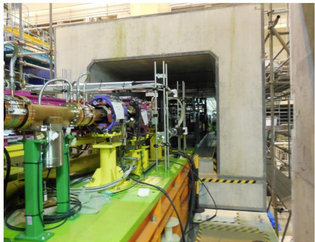
Figure 6: Radiation shield covering the beam line is shown.
