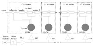
Figure1: Layout of 800 MeV linac of HLS-II.
