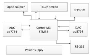
Figure 4: The scheme of ARM-based control module.
