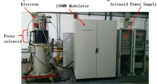
Figure 2: The power supply system of the klystron of HLS-II.
