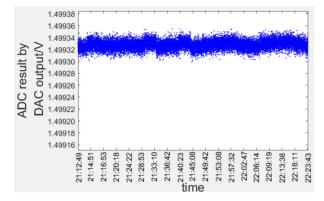
Figure 7: Test result of ADC by DAC output.
