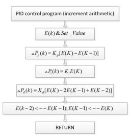
Figure 5: Flow diagram of PID calculation of ARM.
