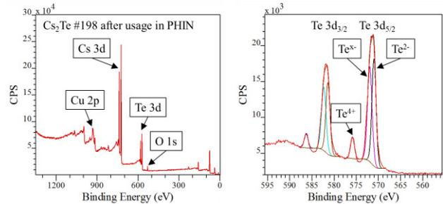
Figure 7: XPS spectrum (wide range and Te region) of cathode #198 after usage in PHIN 2014 [8].
