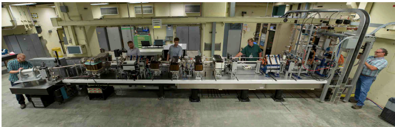
Figure 2: Photograph of X-band test accelerator in the south cave of B194 at LLNL.
