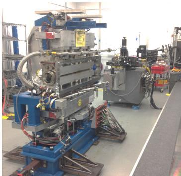
Figure 7: In-Vacuum Undulator X25.
