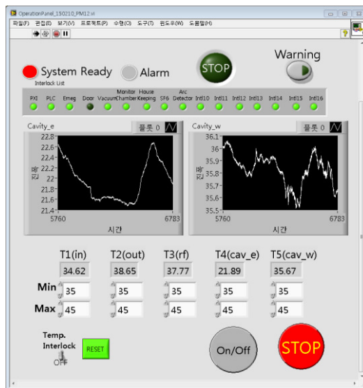
Figure 3: Operation panel in expert mode. (It will not allow for normal operator to use it in the radiotherapy mode.)
