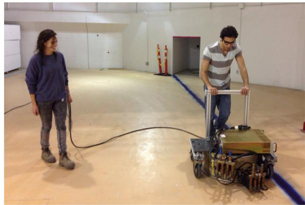
Figure 4: Degaussing coil, on wheels, with a steel plate and a 40 A AC power supply on top. The blue line on the floor indicates the location where the beamline/linac is now installed.
