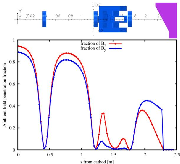
Figure 6: Top: side view of the OPERA model of the low energy transport line, that include 3 solenoids, one dipole (for momentum analysis) and the magnetic shield of the first accelerator cryomodule (magenta).
