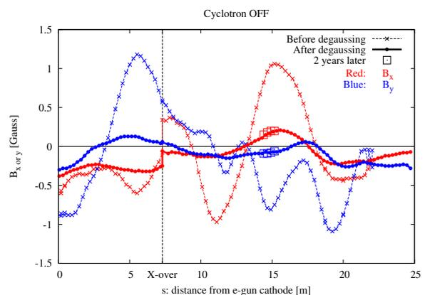
Figure 5: Ambient field measured before (same data as in Fig. 2) and after degaussing the electron hall. A third series of measurements, carried out  $\sim$ two years later on a small section of the beamline shows that the permanent magnetization did not come back.
