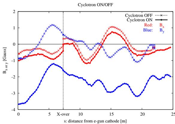
Figure 2: Transverse magnetic field components along the electron beam path ( $B_x$ : horizontal,  $B_y$ : vertical). Data is plotted as is (no smoothing). The discontinuity in  $B_x$  at  $s=7.3$  m corresponds to the point where the coordinate system rotates to follow the beam path. Note: the fluctuations in  $B_y$  observed around  $s = 22$  m have been caused by motion of the overhead cyclotron crane.
