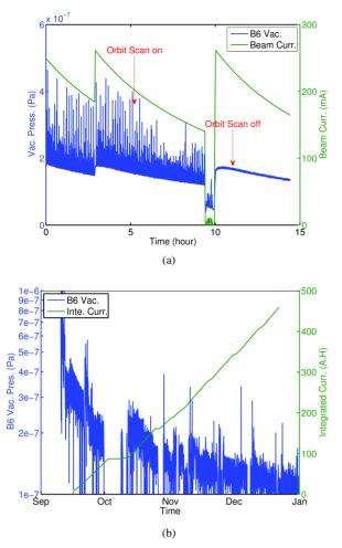
Figure 2: Vacuum scrubbing and recovering at the location of the 6th dipole, B6. (a) Orbit scan for vacuum scrubbing;(b)Vacuum recovering.
