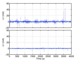
Figure 5: The stability of the PS output at fixed setpoints. (up) before optimization; (down) after optimization.
