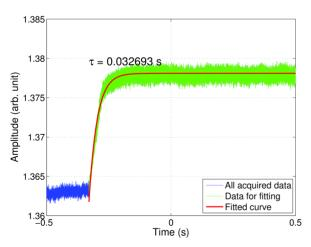
Figure 6: The rising curve of the power supply output.
