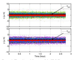
Figure 4: The orbit stabilization of the HLS-II storage ring. All the BPM values and the rms orbit value over all BPMs are plotted as a function of time.
