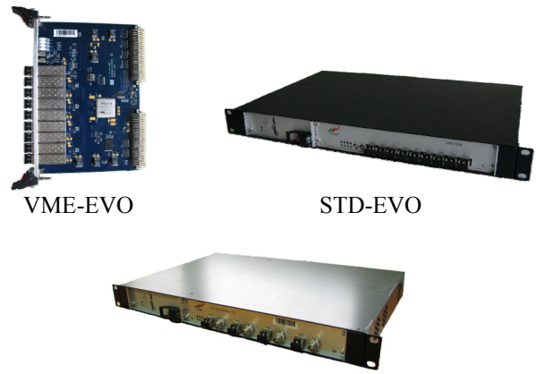
Figure 5: Hardware of timing system in Shanghai Proton Therapy Project.
