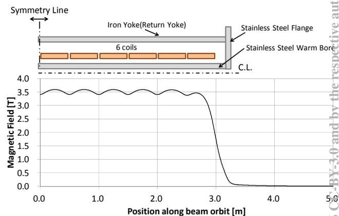
Figure 1: Schematic diagram of the solenoid design and the magnetic field calculation result.
