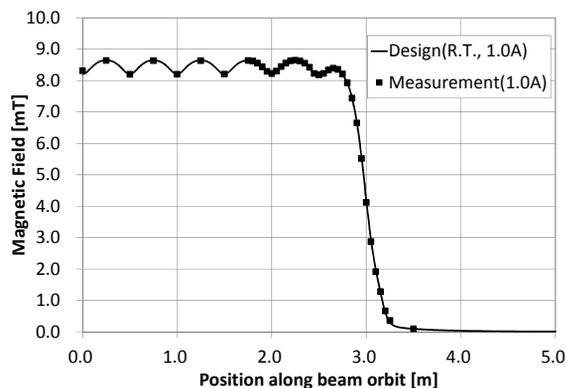
Figure 4: Magnetic field measurement at R.T. in comparison with calculation. This graph indicates the measurement of the beam line downstream region.
