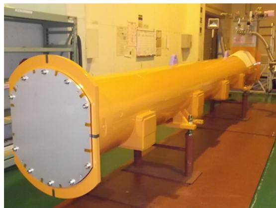
Figure 3: Completion of the Superconducting Solenoid.
