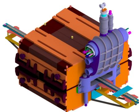
Figure 1: The translating fluxmeter setup in the main Super-FRS dipole.
