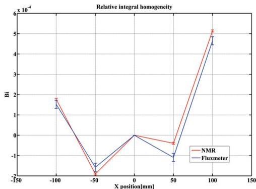
Figure 4: The integral field homogeneity as a function of the transversal position in the magnet.
