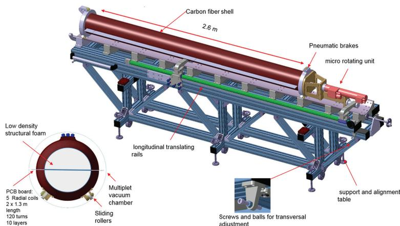
Figure 3: The rotating coil shaft assembly.
