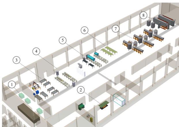
Figure 2: Schematic 3d-view of the facility halls and main equipment placement: 1 – Nuclotron-type SC cable production hall; 2 – magnets windings production hall; 3 –assembling the yoke of the magnet and winding, welding and brazing cooling channels of magnets; 4 –room temperature magnetic measurements; 5 –check vacuum tightness of cooling channels, beam pipes and cryostats; 6 –assembling magnets in cryostats; 7 –cryogenic tests of magnets at 6 benches; 8 –power converters hall.
