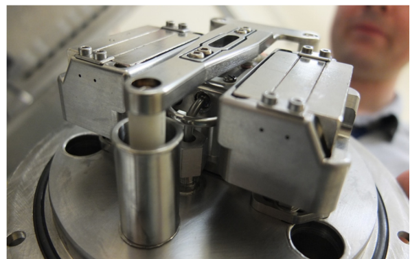
Figure 2: Scaled source mounted on the flange with Nd 2 Fe 14 B permanent magnets for Penning field and extraction electrode with support insulators.
