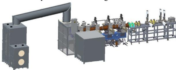
Figure 1: Schematic view of the BTF. Ion source, RFQ, and MEBT from left to right.
