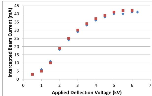
Figure 3: Beam currents in the range of 40-45mA have been measured from a baseline SNS ion source which is within expectation for that particular ion source.
