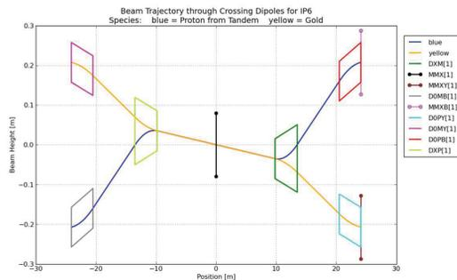
Figure 1: The orbits at STAR experiment in p-Au run. The Blue and Yellow beams collide head-on with a common angle of 3.62 mrad. The two magnets closer to IP (at 0 m) are the common DX magnets. The other four are the D0 magnets.
