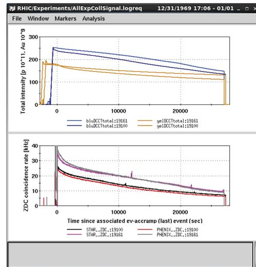
Figure 3: The impact of proton injection working point on the experiments collision rates. The beam intensities for fill 19100 and 19161 are the same. The working point for fill 19161 was at nominal (0.695, 0.692). The working point for fill 19100 was at (0.6926, 0.6898).
