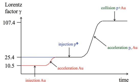
Figure 2: The acceleration cycle for p-Au. The Au beam is injected at  $\gamma = 10.5$ . It is accelerated above transition to  $\gamma = 25.4$  during a mini-ramp. While the Au beam sits on the porch, the polarized proton beam is injected with matched frequency. Then both beams are accelerated to top energies.
