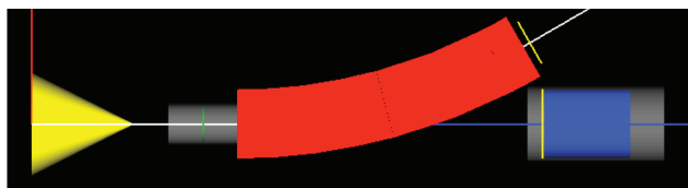
Figure 6: The radiator portion of an energy-recovery linac for radioisotope production. The electron beam emanates from the yellow cone, hitting the gamma production target (green) inside a beam pipe (gray); the charged particles are bent by the magnet (red), while the gammas exit through a hole in its side along the blue line to the production target (blue).
