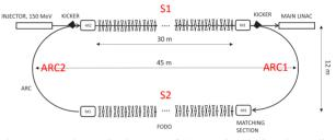
Figure 1: Schematic layout of the recirculating beamline (not to scale), from Ref. [10].
