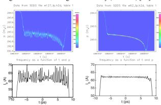
Figure 6: (Top) the longitudinal phase-space distributions at the end of the beamline for Case (i) (left) and Case (ii) (right); (bottom) the bunch current profile for case (i) (left) and (ii) (right).
