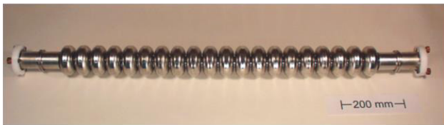
Figure 4: Picture of a S-DALINAC 20 cell cavity.
