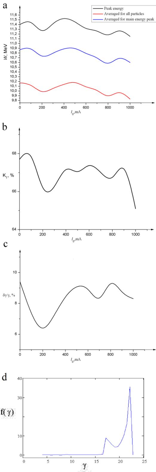
Figure 1: Output beam energy  $W$  (a), current transmission coefficient  $K_T$  (b) and output energy spectrum measured for full width  $\delta\gamma/\gamma$  on the distribution base (c) vs. injection current ( $E_{max}=200$  kV/cm) and typical beam energy spectrum (d) for  $E_{max}=200$  kV/cm.
