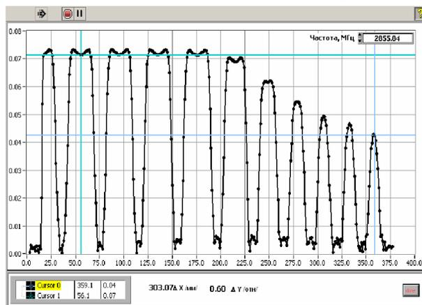
Figure 2: Measured RF field distribution in buncher and first regular cells, the amplitude deviation is not exceeds of 5 % from the simulated one.
