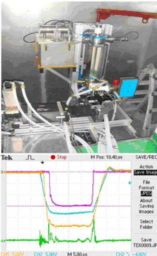
Figure 3: Photo of assembled linac (it is installed vertically over the conveyer) and experimental curves for klystron voltage pulse (yellow), E-gun pulse (cyan), beam pulse (magenta) and reflected RF wave (green).
