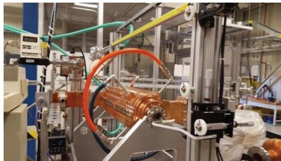
Figure 2: T-cavity tuning setup.
