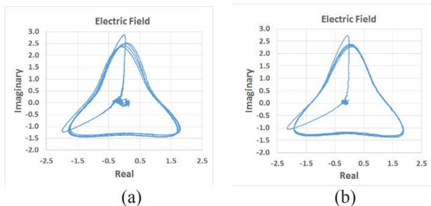
Figure 3: Plots of the complex-valued electric field: (a) cavity tuned such that LRC is reduced to specifications and (b) cavity fine-tuned to compensate for unequal tuning of neighboring cells.
