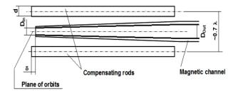
Figure 6: The extracting system of the L-band microtron.
