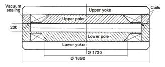
Figure 5: Sketch of the 9.5 MeV tubeless generic microtron magnetic-vacuum system. All sizes are in mm.
