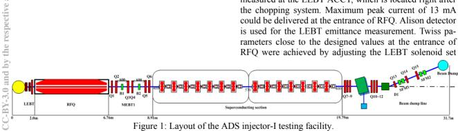
Figure 1: Layout of the ADS injector-I testing facility.
