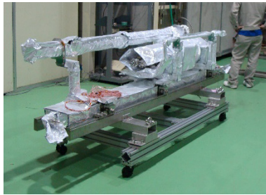
Figure 3: The L-band 9-cell cavity before installed into the cryostat. It has the He jacket and two phase He pipe.
