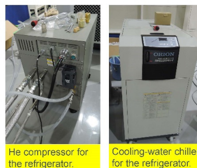
Figure 2: Left-hand side: a picture of He compressor for the refrigerator tube. Right-hand side: a picture of cooling-water chiller for the He compressor.
