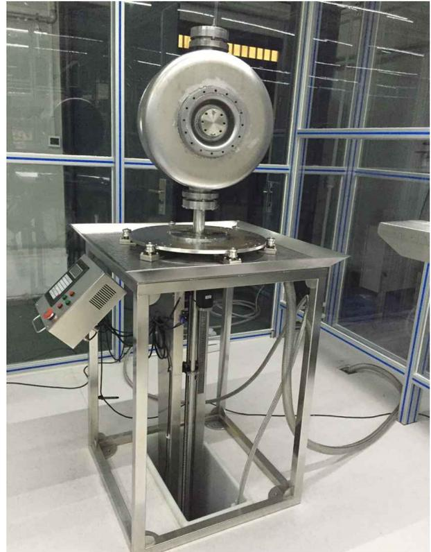
Figure 4: High pressure rinsing facility at IHEP.
