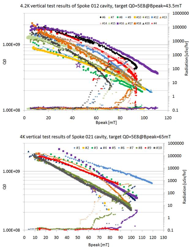
Figure 5: vertical RF test results of spoke 012 and 021 cavities.
