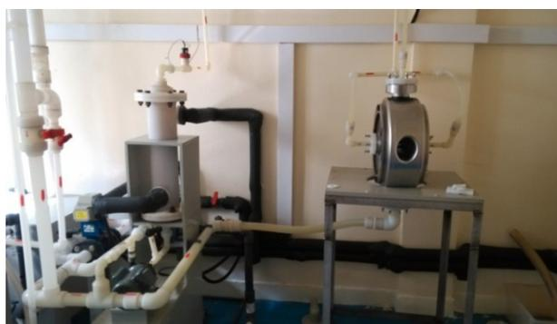
Figure 1: Buffered chemical polishing system.
