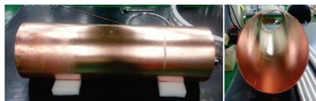
Figure 3: The out conductor made of OFHC for attaching niobium samples, front view (left), side view (right).
