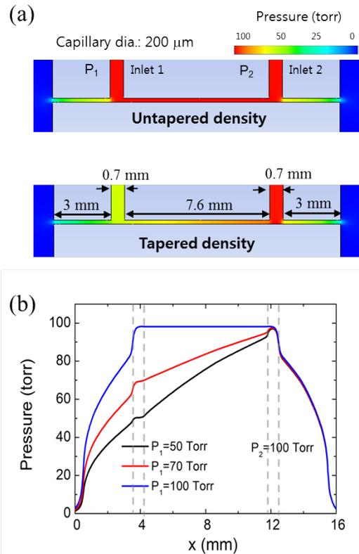
Figure 1: (a) Pressure distribution of a capillary depending on backing pressures at both inlets. When the different pressures are injected through each inlet, the density gradient is produced inside the capillary. (see lower figure) (b) The lineouts along the capillary axis with different  $P_1$  under the backing pressure of  $P_2 = 100$  Torr. The two dash lines indicate inlet positions.
