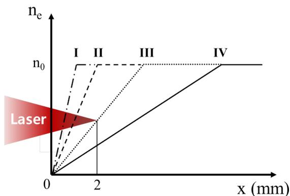
Figure 2: Schematic of the tapered plasma density profile for PIC simulation. Focal point of the laser pulse is fixed at  $x=2$  mm and the up-ramp density distance  $d_R$  varies from 1 to 7 mm (I:  $d_R = 1$  mm, II:  $d_R = 2$  mm, III:  $d_R = 4$  mm, IV:  $d_R = 7$  mm).
