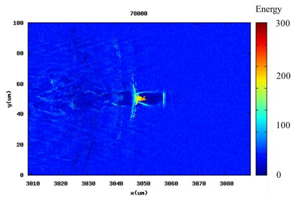
Figure 3: Electron bunch accelerated to high energy ( $\sim 300$  MeV) by a tapered plasma density profile.
