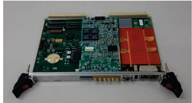
Figure 2: Digital LLRF PMC board and VME board.
