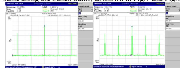
Figure 7: Sidebands on the spectrum when LFB turns on or off.
