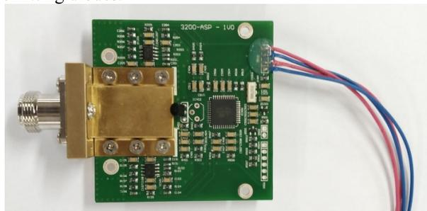
Figure 3: A power detector.
