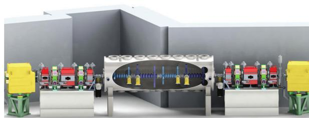
Figure 2: Schematic view of the BESSY VSR cavities straight with the cryo module.
