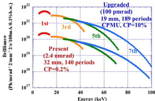
Figure 3: Comparison of undulator radiation spectra between upgraded and present SPring-8.
