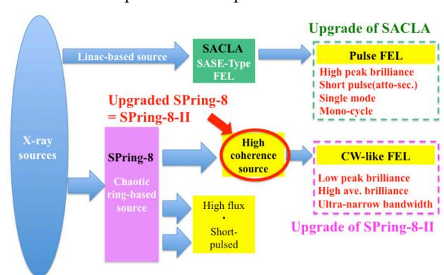
Figure 1: Schematic chart of X-ray source evolution and the SPring-8's strategy for the light source upgrade.
